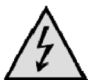
Figure 1 -- High-voltage warning mark
